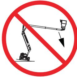
**NEVER** elevate the platform or drive the machine while elevated unless the machine is on a firm, level surface.
