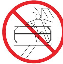
**NEVER** position the platform without first checking for overhead obstructions or other hazards.
