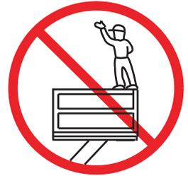
**NEVER** climb, stand, or sit on platform guardrails or midrail.
