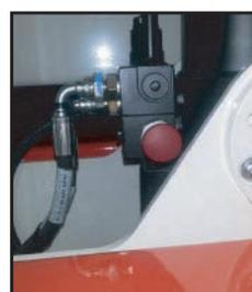
**Before operating the Emergency Lowering Valves the surrounding area should first be cleared of any potential obstructions. It is also important that when the valve is pushed, it is initially done slowly. This is so that sudden movement will not occur in the Elevating Assembly, leading to a potentially unstable machine.**
