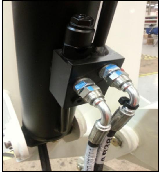
*The Overcentre Valves are located towards the Rod End of the Lower Lift and Upper Lift Cylinders.*
