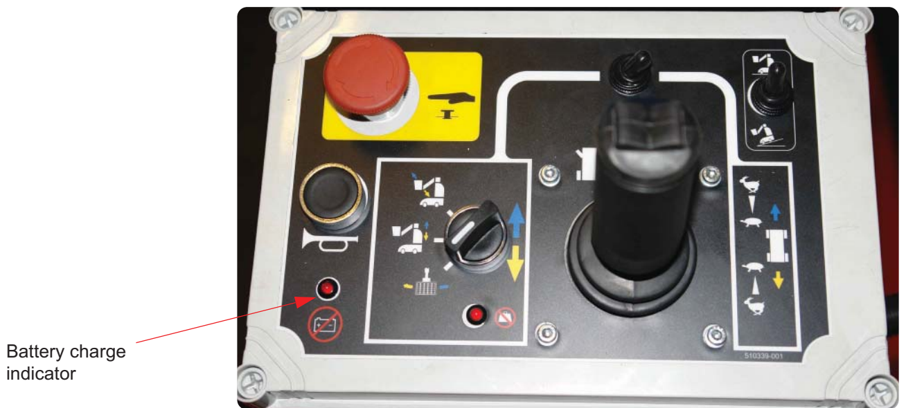
Figure 3-30: Upper Control Panel with Battery Indicator
