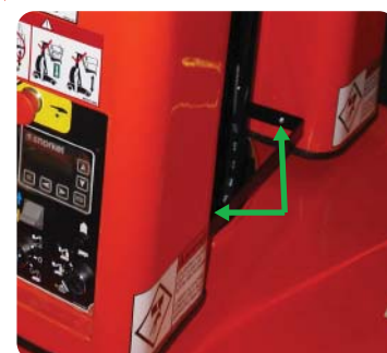
Figure 3-8: Mast Cover Removal
