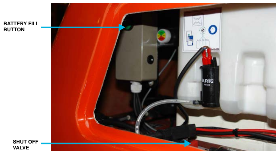
Figure 3: Battery Fill Button & Valve
