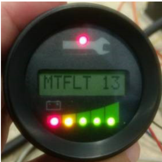
Motor Fault Display
