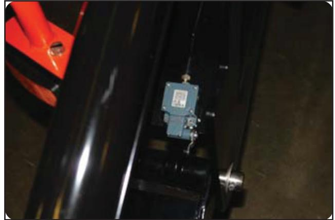
Figure 3-27: Outrigger limit switch.
