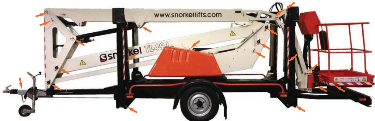
Figure 3-35: General grease point locations.
