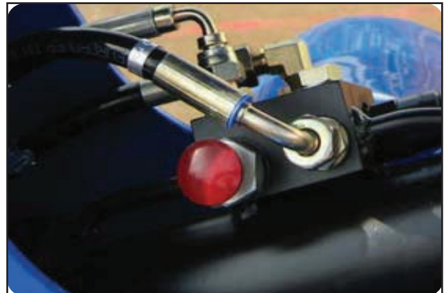
Figure 3-29: Emergency lowering valve.
