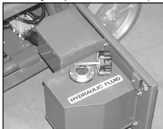
Figure 9: Hydraulic Fluid Reservoir and Dipstick
