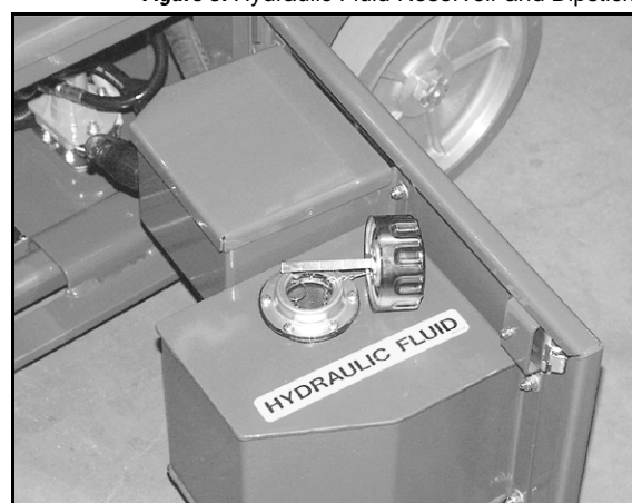
Figure 8: Hydraulic Fluid Reservoir and Dipstick
