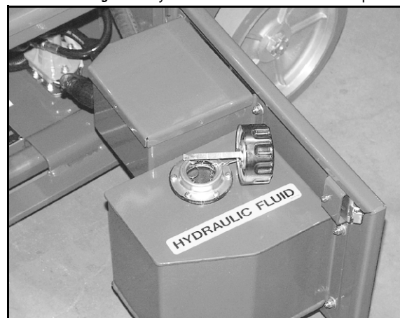
Figure 8: Hydraulic Fluid Reservoir and Dipstick
